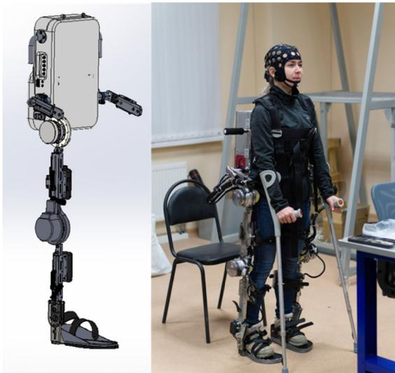
**FIGURE 4.** Laboratory setup of the lower-limb exoskeleton integrated with mHMI.
