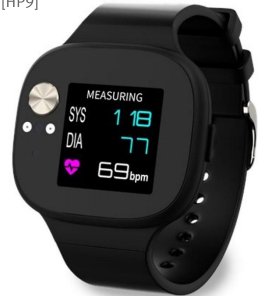
ASUS Vivo watch for ECG, PPG and thus blood pressure estimation (2018)
